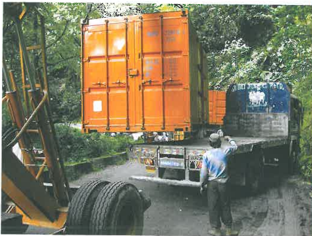
Shaft Sinkers' contract for the Teesta III hydro-electric scheme has been complicated by difficult access to the site with trucks sometimes having to be offloaded and reloaded to allow them to negotiate rock overhangs on the route (photo: Shaft Sinkers).
